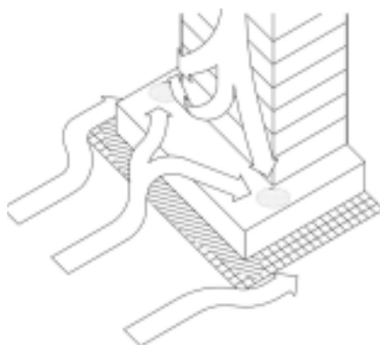
Figure 10: The tower-on-podium massing often results in reasonable conditions at ground level, but the podium may not be useable.
