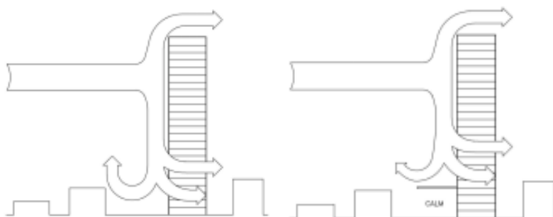
Figure 9: Canopy Windbreak Treatment. (L) Downwash to street level may generate windy conditions for pedestrians. This is particularly true for buildings much taller than the surrounding buildings. (R) A large canopy is a common solution to this pedestrian-wind problem at street level.
